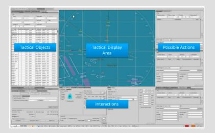
To provide optimum support for the duties of the operator, the information content of the user interface is adapted to fit the specific role of the operator. The layout of the display always follows the same system. Here too, the interface exhibits a modular structure.
